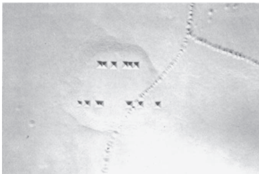
FIG. 5.3 The large square etched pits in horizontal rows correspond to dislocations formed in LiF at room temperature, while the smaller, closely spaced pits lying in curved rows were grown into the crystal when it was manufactured (Gilman, J. J., and Johnson, W. G., Dislocations and Mechanical Properties of Crystals , p. 116, John Wiley and Sons, Inc., New York, 1957. Used by permission of the author.)
