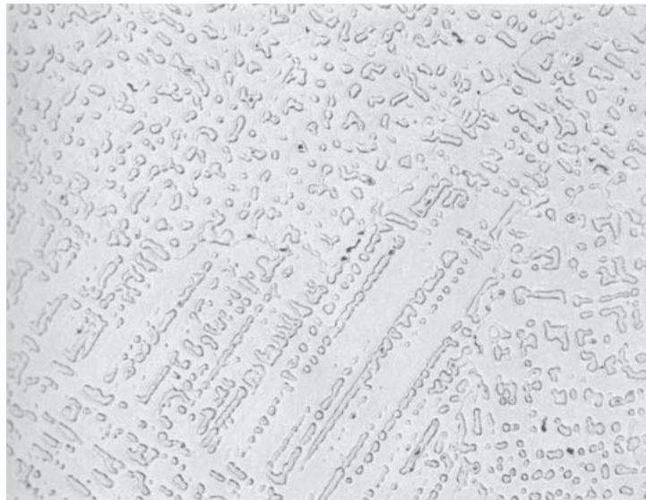
FIG. 14.34 Coring, or dendritic segregation, in a copper-tin alloy. Several different grains are shown. Note that the dendrite arms have different orientations in each crystal. 200X
