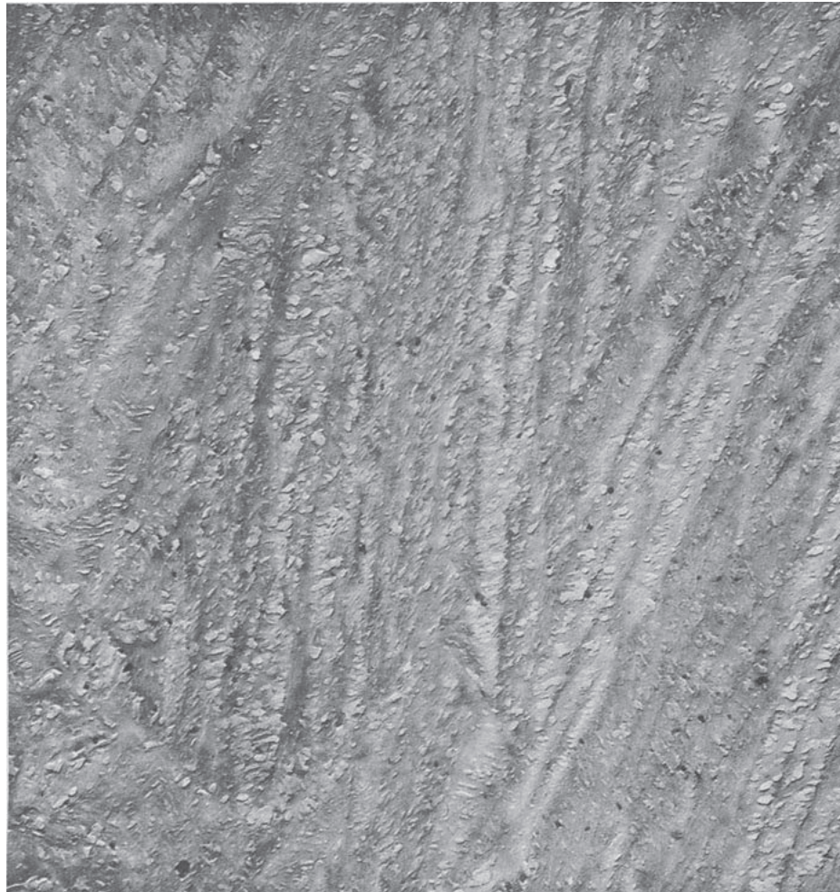
FIG. 18.27 The structure of bainite transformed at 523 K (250°C) as revealed by the electron microscope. Original magnification 15,000 \times reduced 30 percent in above photograph. ( Trans. ASTM , 50 , 444, Fig. 23 [1952]. [Second Progress Report of Subcommittee XI of Committee E-4]). Copyright ASTM International. Reprinted with permission.
