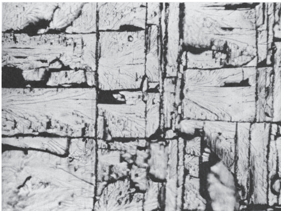
FIG. 21.7 Cleavage-fracture surface of an iron crystal. (Reprinted from Biggs, W.D., and Pratt, P.L., "The deformation and fracture of alpha-iron at low temperatures" Acta. Met. , 6 (11) 694 [1958] with permission from Elsevier.)
